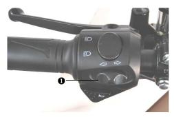
The steering lamp switch **①** is on the left handle switch.
