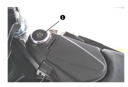
Start/stop button is used to start or stop the motorcycle.
