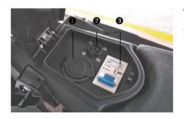
The main circuit breaker **3** is the protection switch of ES1 PRO main power supply. When the current caused by abnormal or short circuit of the motorcycle exceeds the safety setting value, the air switch will be automatically disconnected to ensure safety.
