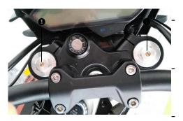
The hydraulic rebound damping system determines the performance of the front suspension when it bounces up.
