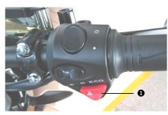
When the button • is pressed, the turning lights flash to warn other drivers of situations, which include stop or park under emergency conditions.
