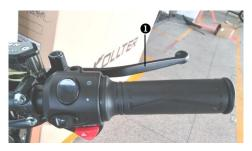
The front brake handle **①** is fitted on the right side of the handlebar.
