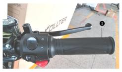
The throttle grip **①** is fitted on the right side of the handlebar.
