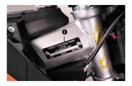
The nameplate **①** is mounted on the chassis at the front right.
