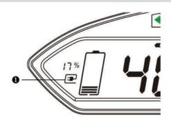
During cycling, when you brake the vehicle, the controller recovers the braking energy. At the same time the charging symbol will light up.
