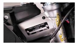
The chassis number **①** is stamped on the right side of the steering head.
