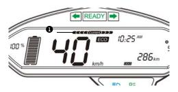
The current indication • displays the real-time current in the form of a status bar. You can roughly determine the current real-time current through the status bar
