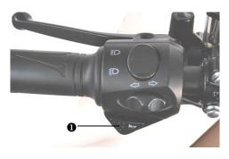
When the key is in the ON position, the horn sounds when the button **①** is pressed. the horn can be used to warn pedestrians or other motorists of your presence.
