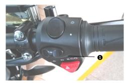
The driving mode switch ① is on the right handle switch.
