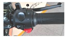
Flip the switch upward to  $\heartsuit$ , open the Headlight. Flip the switch down to  $\bullet$ , open the Headlight.
