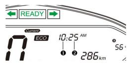
Press and hold the adjustment button at the back of the instrument panel, then switch on to enter the setting interface.
