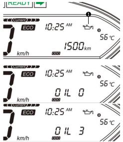
According to the mileage and time of your trip, the system will automatically remind you that gear oil in the reduction gearbox should be replaced. You can manually clear the reminder after changing the oil, or our service personnel can clear it for you.
