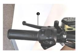
The rear brake lever **①** is fitted on the left side of the handlebar.
