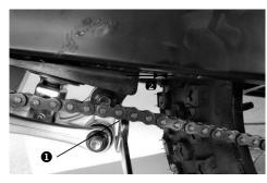
Push the chain at the lower end of the chain support • upward to check the tension of the chain between the chain and the chain support.
