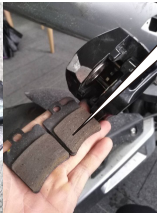
Image 47 Pull out the brake pads
