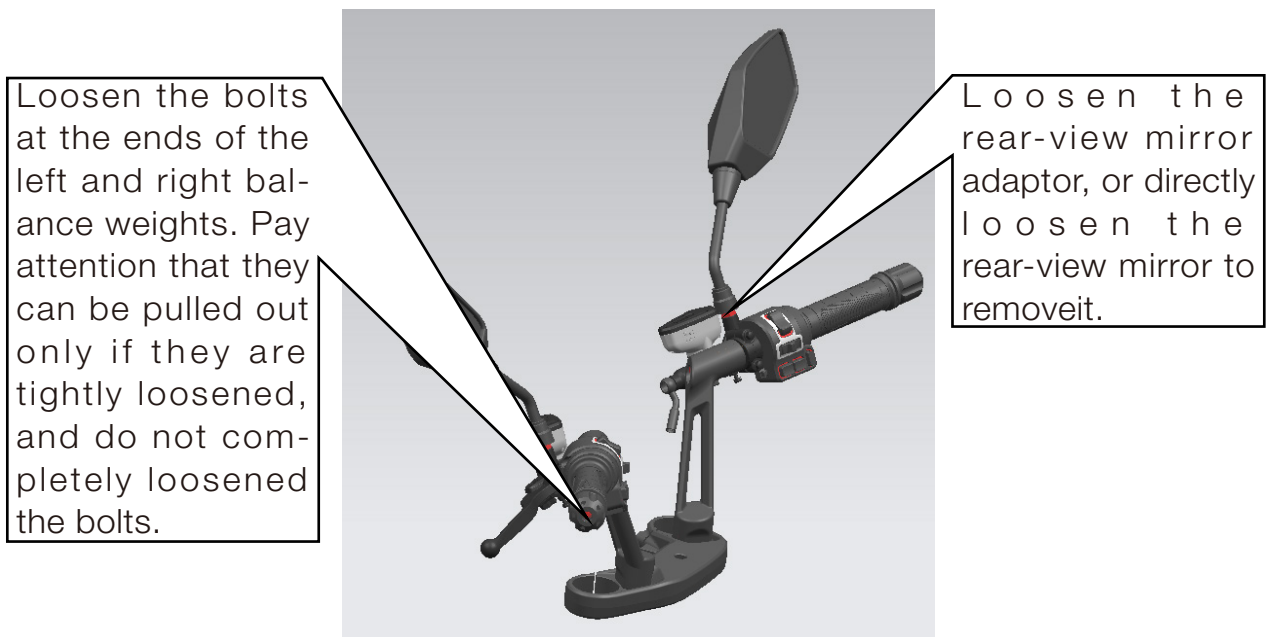
Image 11 Disassemble the balance weight and rearview mirror
