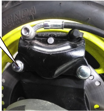
Image 45 Disassemble the bolts
